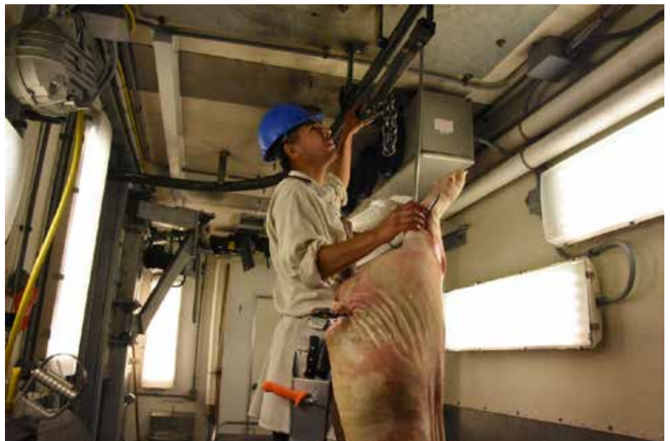
Above: the carcass is pushed into the mobile unit by overhead rail; below and bottom: inside docking station: hot water, electricity, ...
